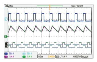
Ultra-high fidelity: magenta: real boost MPPT converter current; green: HIL boost current; dark blue: real boost inductor voltage; light blue: HIL inductor voltage.
